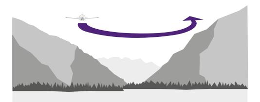
Consider your airspeed and ground speed – the higher your airspeed the greater the turn diameter will be for the same bank angle. At 100 kts and with a  $30^{\circ}$  angle of bank, the turn diameter will be approximately 0.5 NM. Halving the angle of bank to  $15^{\circ}$  would approximately double the diameter to 1 NM.
