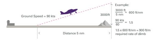
In many light aircraft, an average of 900 ft/min over a 3,000 ft climb will not be achievable, and an alternative route must be found. If the terrain allows, one option may be to climb in an orbit. This will reduce the rate of climb but allows height to be gained while staying in the same area. However, orbiting brings other risks, such as disorientation, midair collision, or failure to monitor airspeed if you are focused on the ground.
