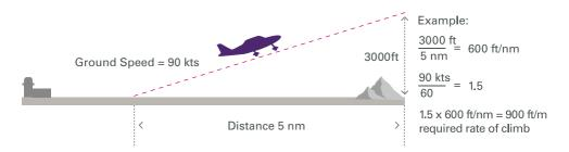
In many light aircraft, an average of 900 ft/min over a 3,000 ft climb will not be achievable, and an alternative route must be found. If the terrain allows, one option may be to climb in an orbit. This will reduce the rate of climb but allows height to be gained while staying in the same area. However, orbiting brings other risks, such as disorientation, midair collision, or failure to monitor airspeed if you are focused on the ground.
