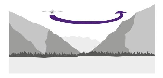
Consider your airspeed and ground speed – the higher your airspeed the greater the turn diameter will be for the same bank angle. At 100 kts and with a 30° angle of bank, the turn diameter will be approximately 0.5 NM. Halving the angle of bank to 15° would approximately double the diameter to 1 NM.
