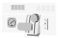
Power changes should be smooth and gradual. Long climbs may put additional strain on the engine. Monitor temperatures and pressures to ensure they remain within limits. If oil or water temperatures begin to rise above normal, you may need to lower the nose to increase airflow over the engine or radiator.
