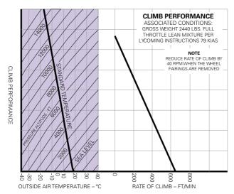
The example graph is referenced to maximum take-off weight (MTOW) – data for lighter weights may not be provided. You will see that at sea level, the rate of climb is around 600 ft/m. Note how the rate of climb decays with altitude.
