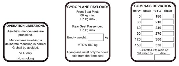
Note: (914UL/915iS MTOM shown, MTOM is 500 kg for aircraft equipped with 912ULS engine)
