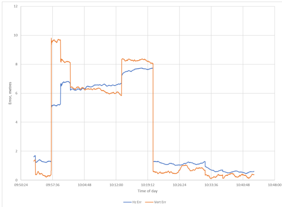
Figure 5-5: Position Error during period of High PRN01 Error on 10 th July 2023 at NOTT
