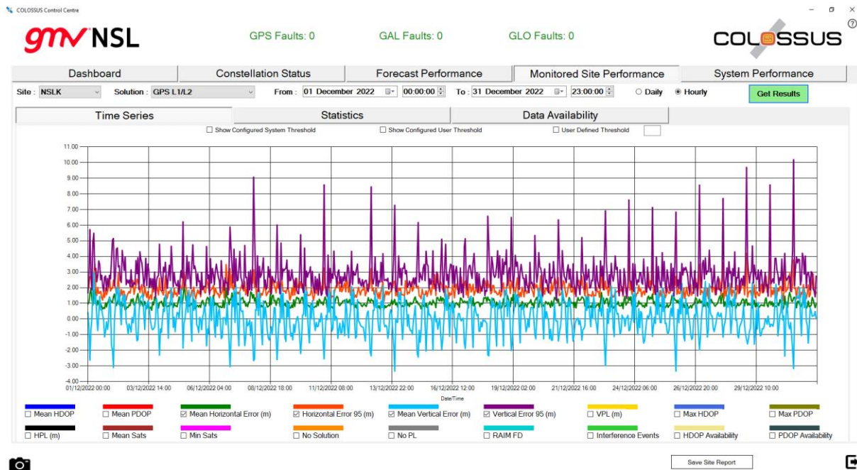
Figure 5-6: Hourly Horizontal and Vertical Error Statistics for GPS L1/L2 during December 2022
