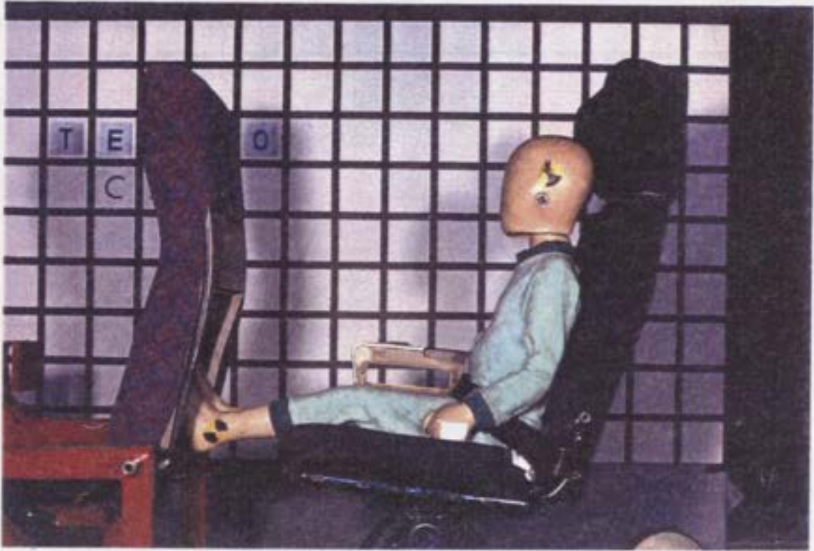
Figure 8 6 year child dummy restrained with an adult lap belt
