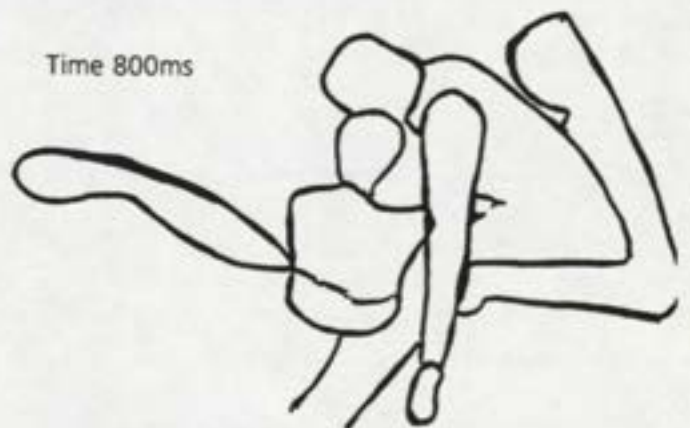
Figure 10 Kinematics of unrestrained, lap held 3 year child dummy
