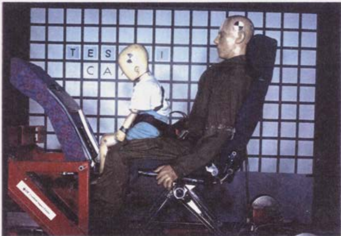
Figure 5 Forward movement allowed by attachment of supplementary belt to adult lap belt
