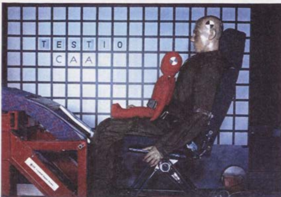
Figure 6 6 month infant dummy restrained with a supplementary belt
