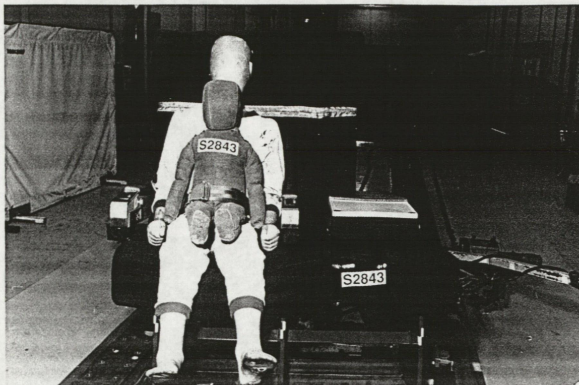
Figure 12 Positions of the 9 month and 10 year dummies on the aircraft seat
