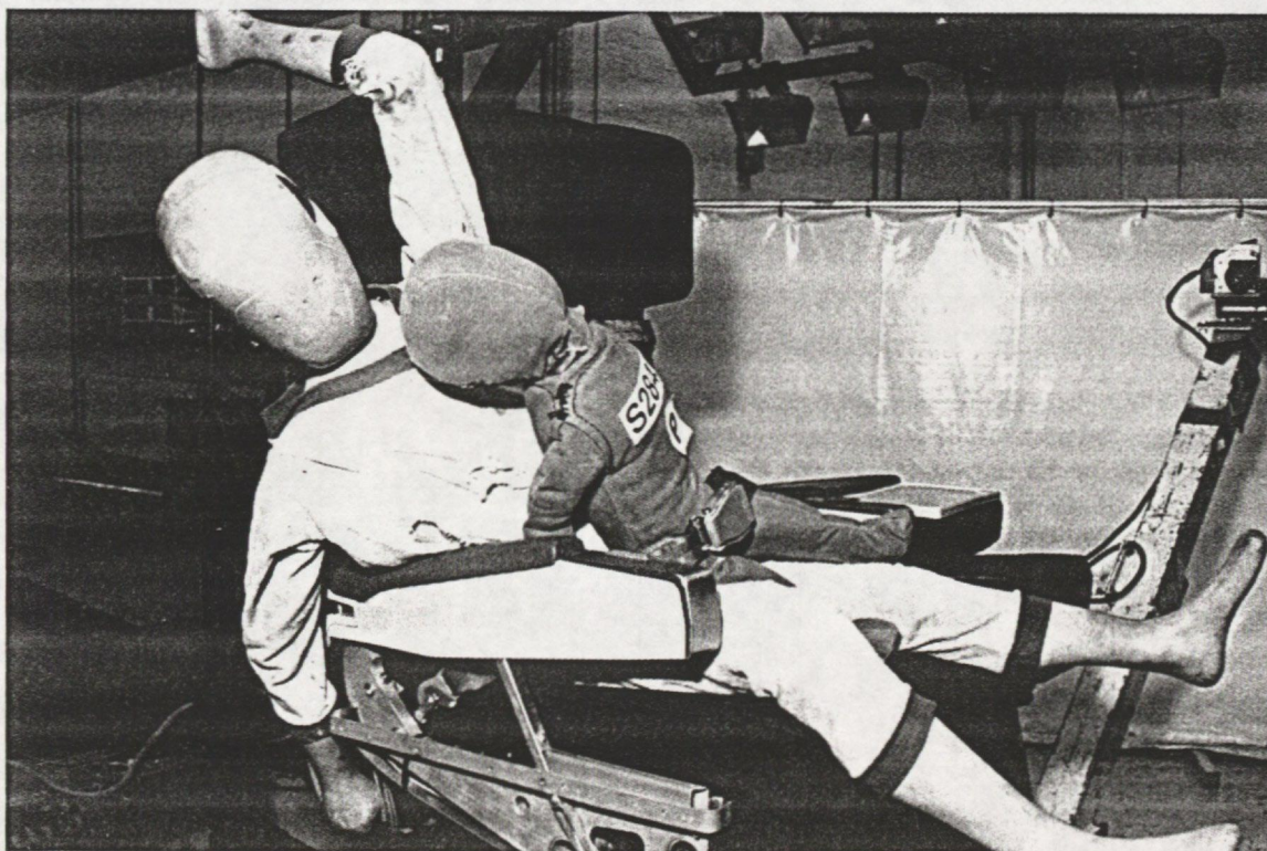
Figure 21a Positions of the 9 month and 10 year dummies after test
