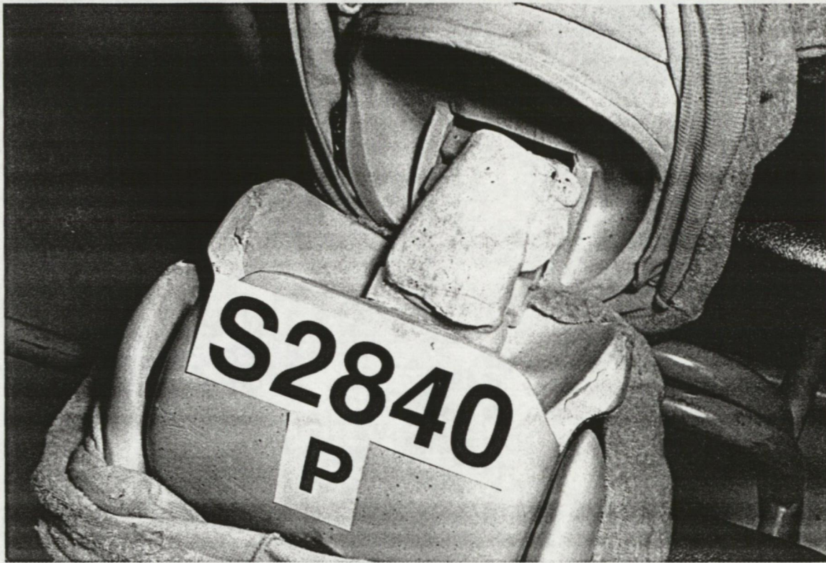
Figure 17b Distortion of plasticine after test
