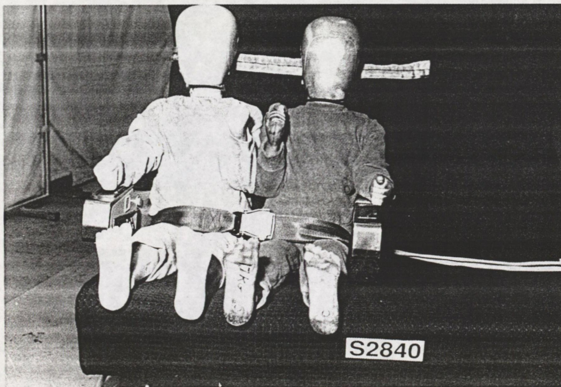
Figure 4 Position of the 10 year dummy on the aircraft seat
