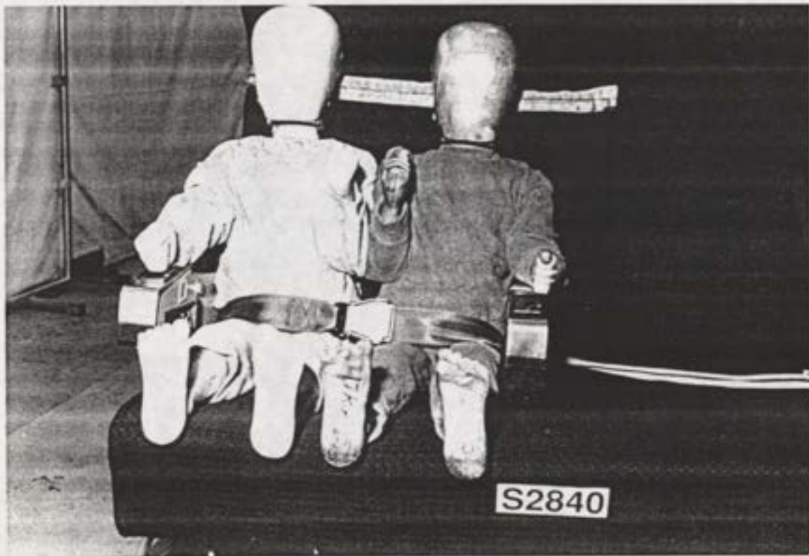
Figure 5 Positions of the two 3 year dummies on the aircraft seat
