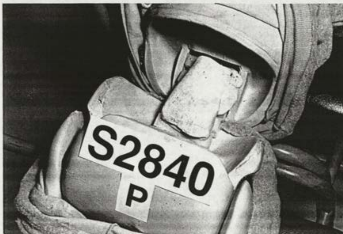
Figure 17b Distortion of plasticine after test
