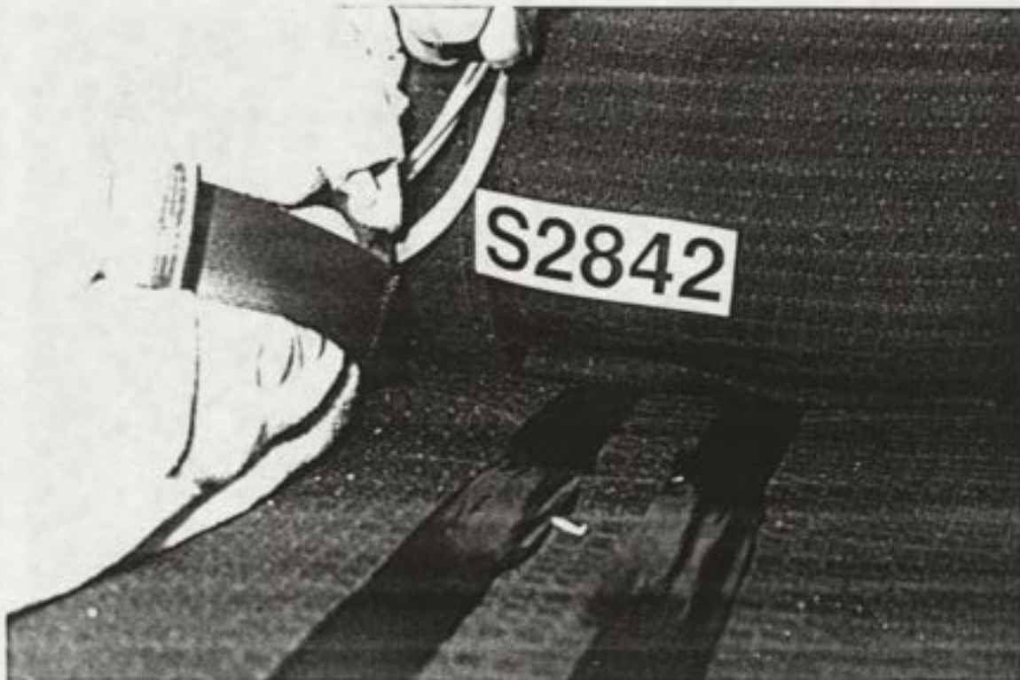
Figure 9 Wrapping of the lap belt around the left hip of the 10 year dummy
