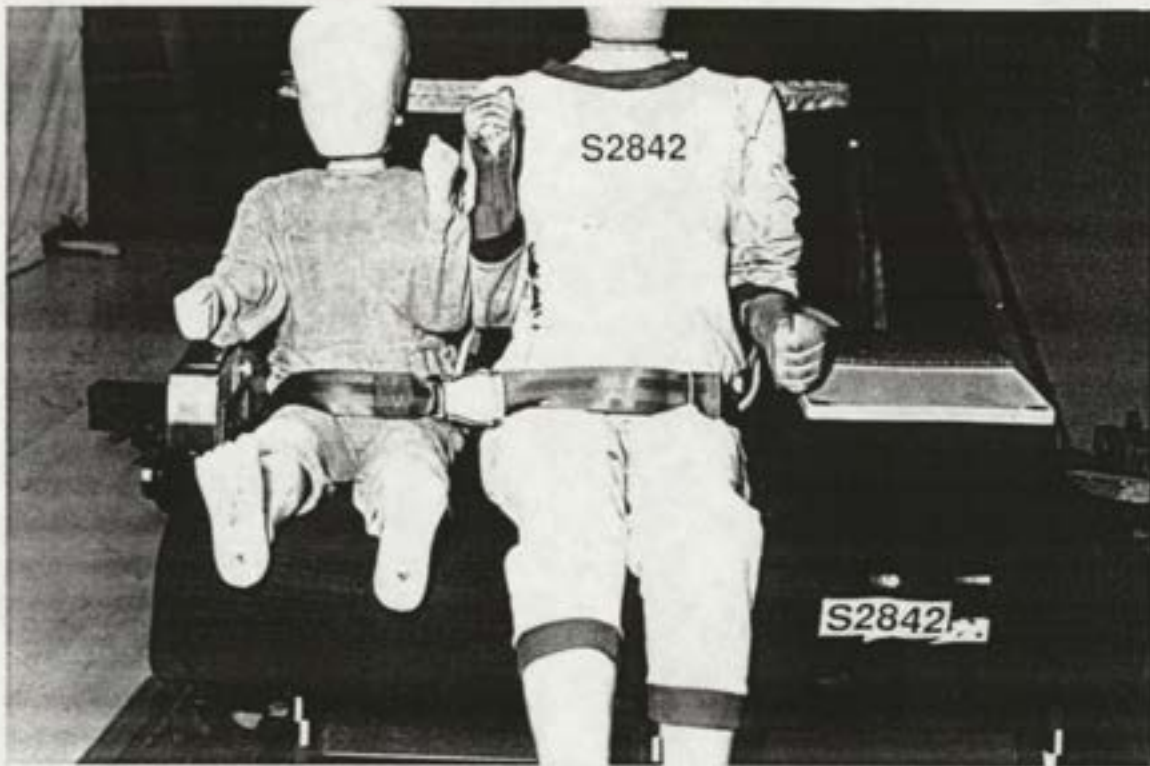
Figure 8 Positions of the 3 year and 10 year dummies on the aircraft seat
