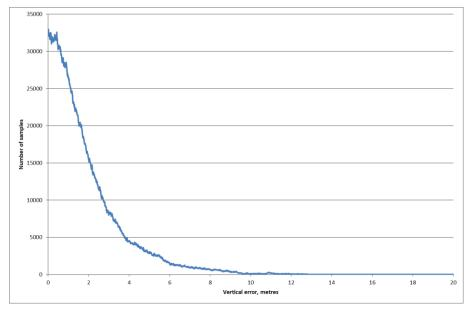
Figure 3-2: Vertical Error Distribution for Monitoring Period
