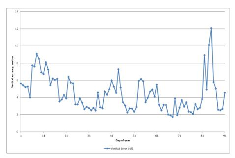
Figure 3-6: Vertical Position Accuracy (95%) for Monitoring Period
