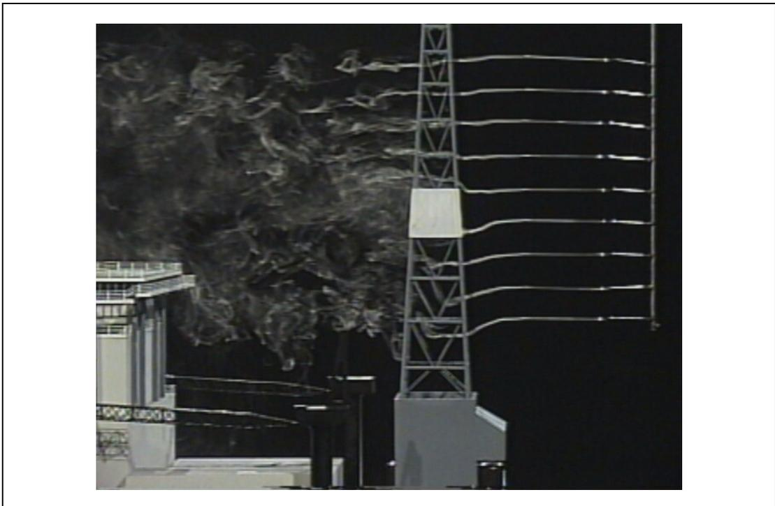
**Figure B-7** Turbulence Created by an Open Lattice Derrick. (Streamers released on the centre of the derrick. Turbulence created by the monkey platform is evident.)
