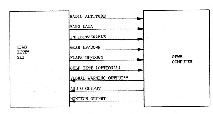
\*SUNDSTRAND - P/N 951-0090-001 BENDIX - CPT-83A COLLINS - 971T-1 EDO - GPW 1501TD LITTON - MODEL GPWS-STC IDC - 28400-001
