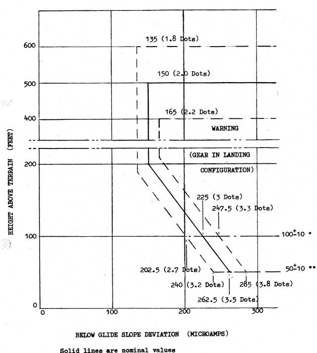
Dashed lines indicate tolerance limits \* Automatic Inhibit Height Upper Limit \*\* Automatic Inhibit Height Lower Limit
